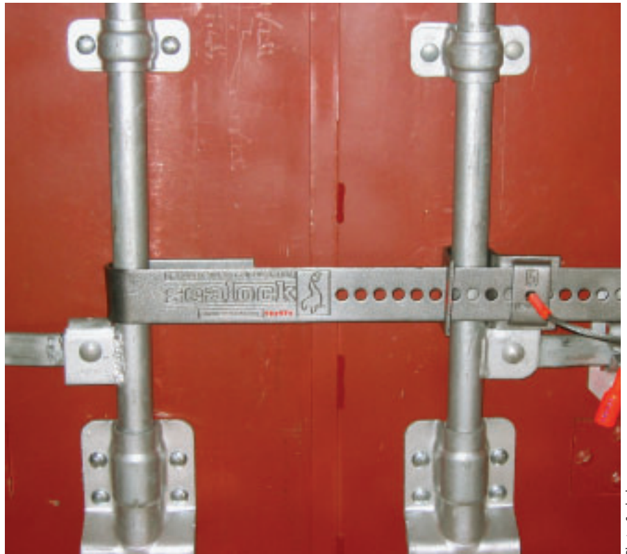
Sealock inventor Jeff Liroff says the combination seal and lock provides greater security because it simultaneously seals the container's locking bars while locking the Sealock into itself.
